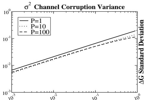
Figure 1: Standard Deviation of  $\Delta G$  vs.  $\sigma_e^2$  for a  $4 \times 4$  System. Power Budgets  $P = 1, 10$  and  $100$  shown.
