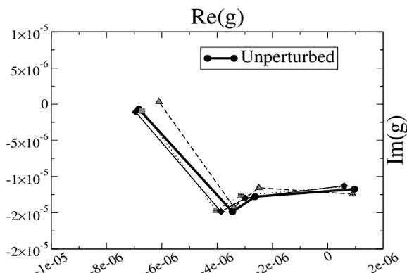
Figure 7:  $2 \times 2$  MIMO Channels Subject to Scatterer Position Perturbation Variance of 0.001 Wavelength. The four gains for each channel instance are connected. Different channel instances are shown with different symbols.
