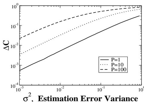
Figure 2: Fractional Capacity Difference  $\Delta C$  vs.  $\sigma_e^2$  for a  $4 \times 4$  System. Power levels as shown.
