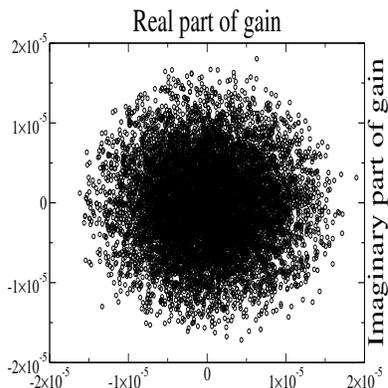
Figure 5: Channel Gain Scatterplot for An 8-Sphere Channel. 1000 trials.
