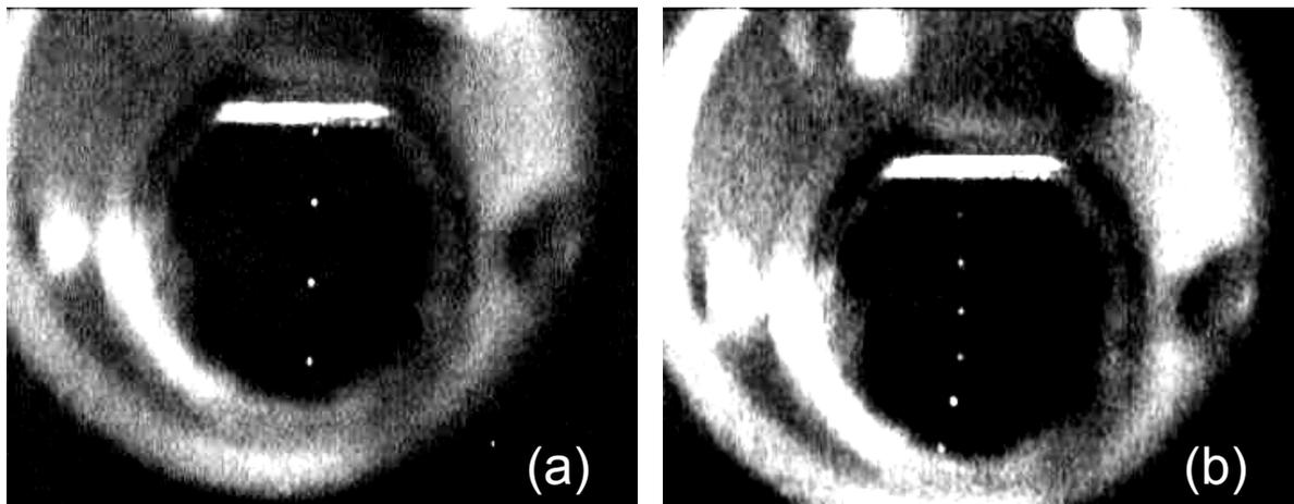
**Figure 2.** Images of electrons moving down the cell. The temperature is 1.35 K in (a) and 1.91 K in (b). The bright horizontal line at the top of each picture comes from light scattered by the holder of the transducer.
