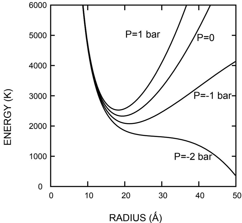
**Figure 1.** The energy of an electron bubble as a function of its radius for several different pressures in the liquid.
